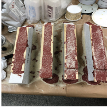
Figure 2: Pull test results for Stonclad UT over Blücher Stainless Steel
