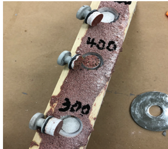
Figure 5: Pull test results for Stonclad UT over PolySto Sanicoat unprepped
