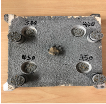
Figure 1: Pull test results for Stonclad UT (top) and Stonclad UR (bottom) over Blücher Stainless Steel
