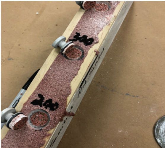
Figure 4: Pull test results for Stonclad UT over PolySto Natural unprepped
